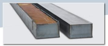
Material & thickness: High-strength steel, 4 mm.
